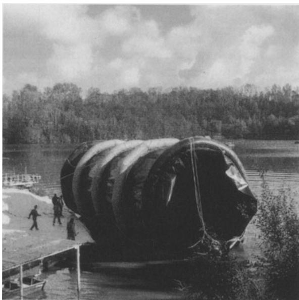
Fig. 20. Installation of an enclosure for sediment investigation in the Schwelvollert deposit in Saxony-Anhalt, Germany (field studies of the UFZ Centre for Environmental Research, Leipzig, photo: (U. Stottmeister)
